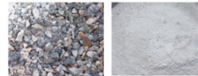
Sample Grinding ball Sample characteristics Attention Time Granite 10mm ball stainless steel Hard Sample no more than 1/4 of total grinding jar 15min
