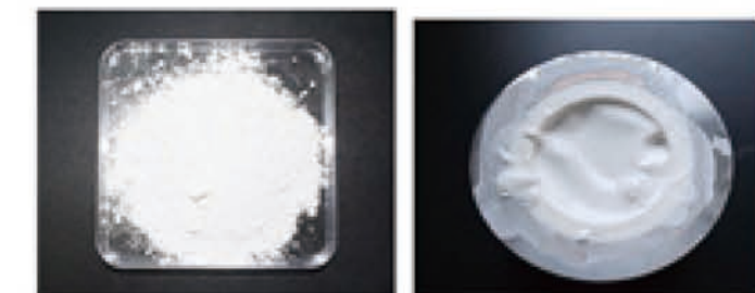
Sample Grinding ball Sample characteristics Attention Time Pearl powder 3mm ball ZrO 2 Brittle Add suitable liquid, ball & sample. Liquid no more than 3/4 of grinding jar. 6h
