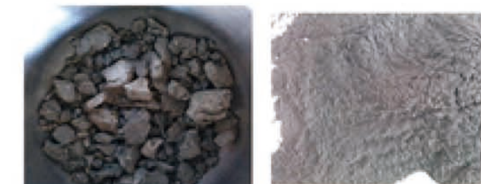
Sample Grinding ball Sample characteristics Attention Time Sludge 10mm ball stainless steel Hard Sample must be dry 35min
