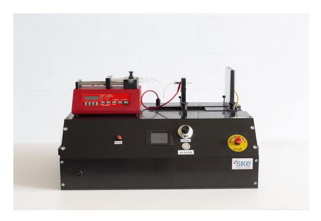
The disposable kit includes 2 stainless steel spinneret of 2 different diameters, 100 syringes, tygon/ptfe tubing (7.5m), polypropylene male and female luer connectors (15+15).
